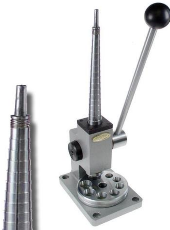
Above, Pepetools Stepped upright ring stretcher. Note the magnified view left showing the stepped mandrel.
